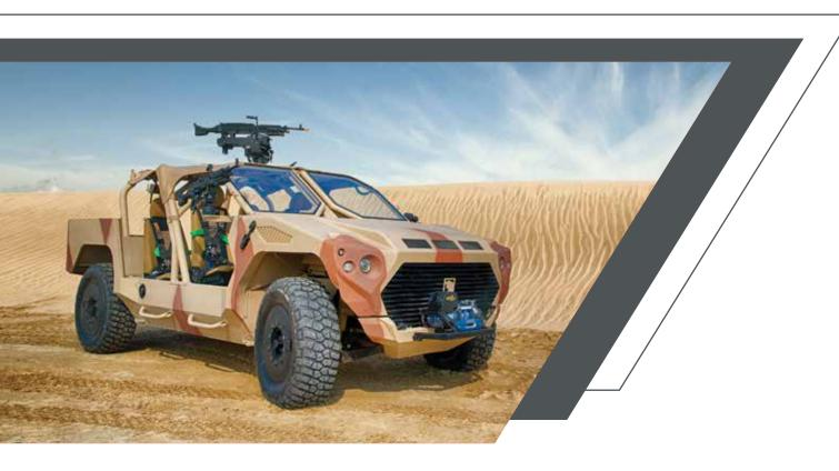
The NIMR Rapid Intervention Vehicle (RIV) is a light 4x4 vehicle, enabling high-speed response to tactical situations in remote sites, either by fast ground transit or helicopter insertion both underslung or inside a CH-47.
